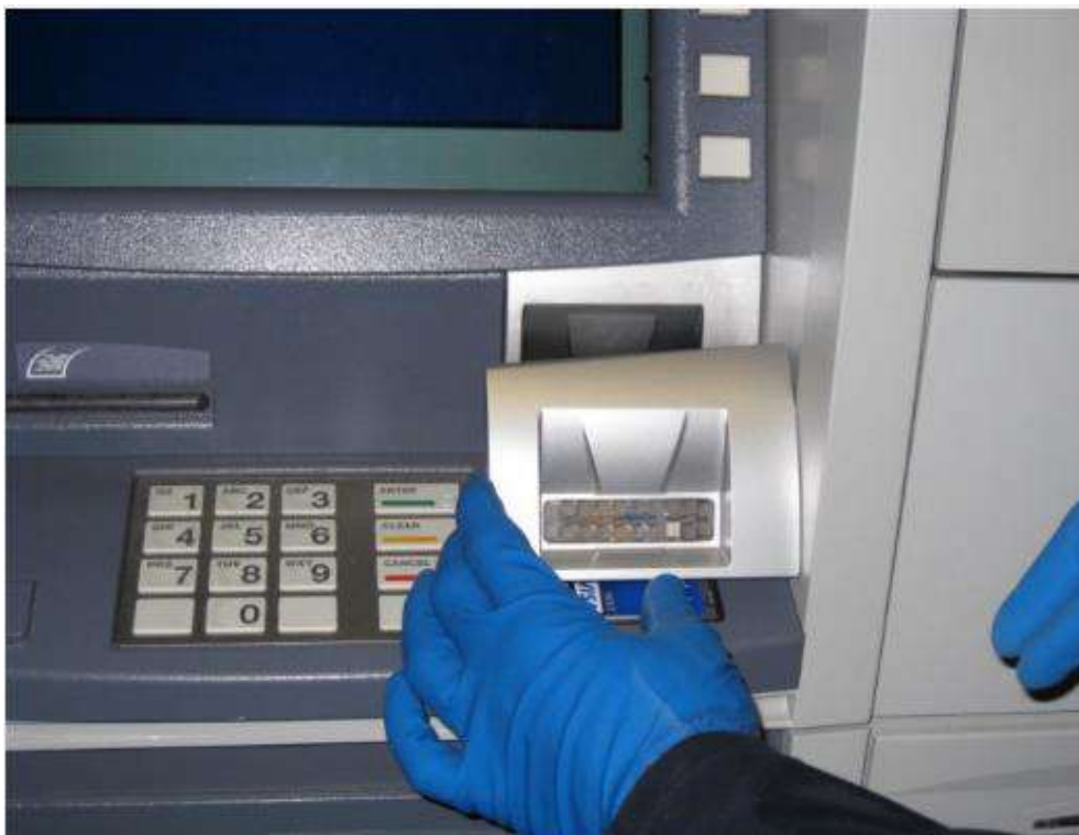
Fig. 4. Skimmer used for ATM
