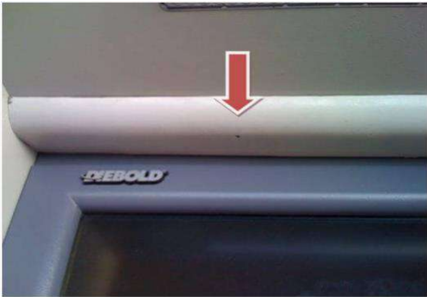
Fig. 3. Hidden camera installed in an ATM
