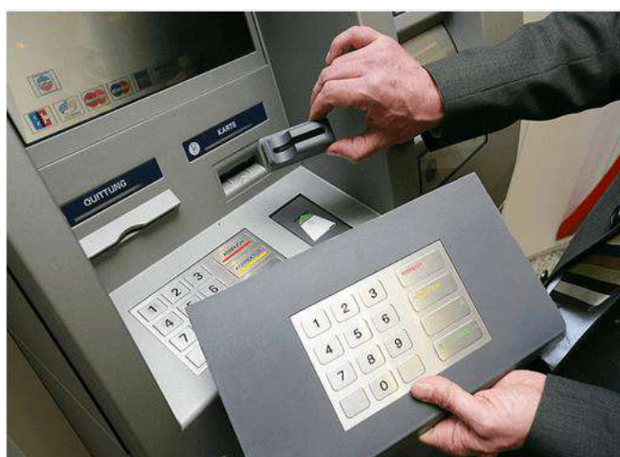
Fig. 1. Pillows, covers for ATM keyboards
